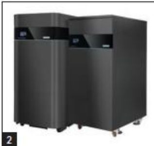
2 Weil-McLain's SVF Commercial Condensing Fire-Tube Boiler features a 316L stainless steel heat exchanger and efficiencies up to 97.1%. Available in six sizes between 750 and 3,000 MBH and fueled with NG or LP. The Unity control system offers programming and an eight boiler sequencer among other features. www.weilmclain.ca
