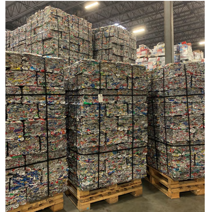
Cans are crushed before shipping to optimize transportation routes and to reduce need for trucks on the road.
