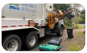
Figure 3-4: RDN automated cart collection truck
