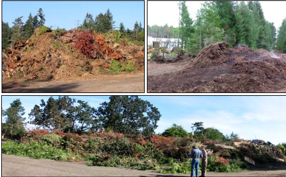
Figure 2 Typical feedstock storage consisting of yard waste, tree and brush trimmings or ground woodwaste. There may be leachate issues associated with feedstock storage. Under the right conditions, fires can break out in the stored materials (note the smoke in the upper right photo).
