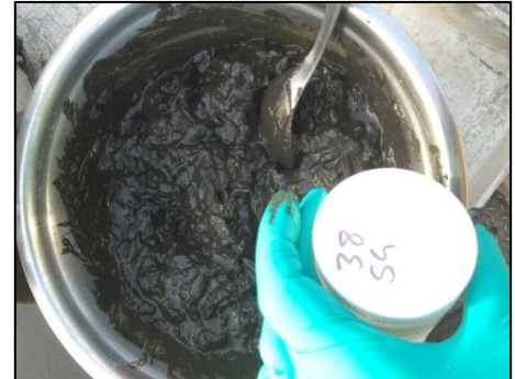
Figure 6: Sediment sample homogenization.
