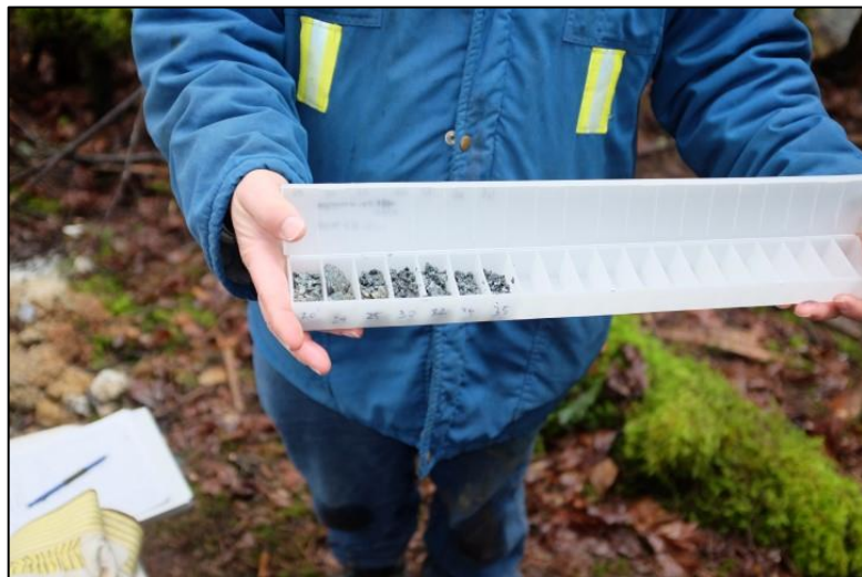
Figure 1.1: Example of a chip tray used to store soil or rock chip samples.
