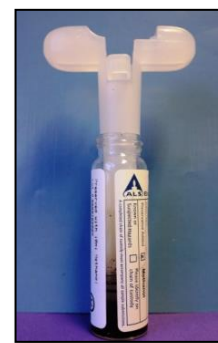
Figure 5. Release of soil plug into a 40 mL vial.
