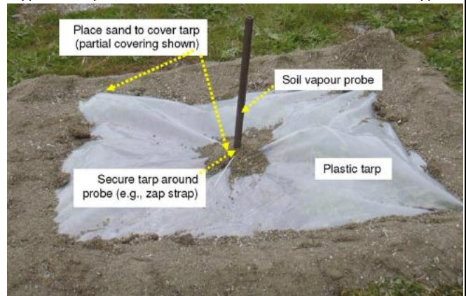
Figure 1. Secured surface seal around soil vapour probe.
