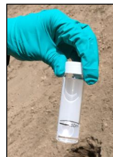
Figure 4. Check methanol fill line.
