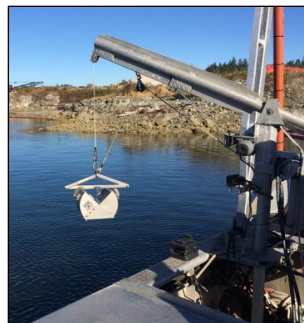
Figure 1: Using a winch/crane system with a Ponar grab sampler (standard size)
