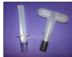
Figure 1. Terra-Core™ with soil plug and syringe samplers
