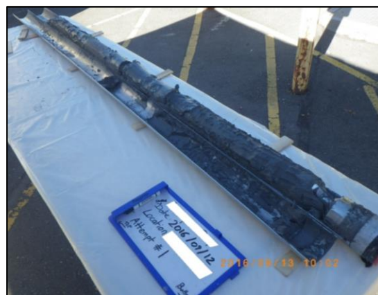
Figure 5: Retrieved sediment core in a stainless steel liner, ready for processing on shore.
