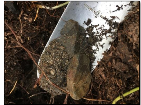
Figure 1. Surficial soil sample collection for soil classification.
