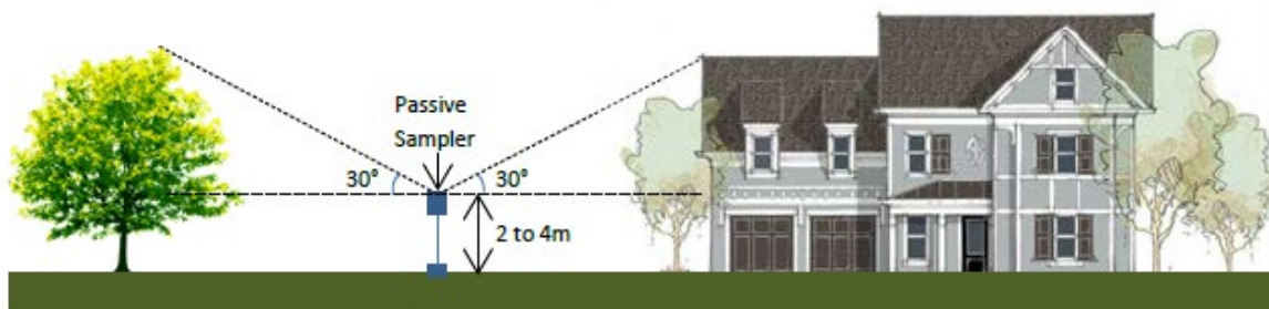
Figure 2.9.1 Passive Sampler Installation
