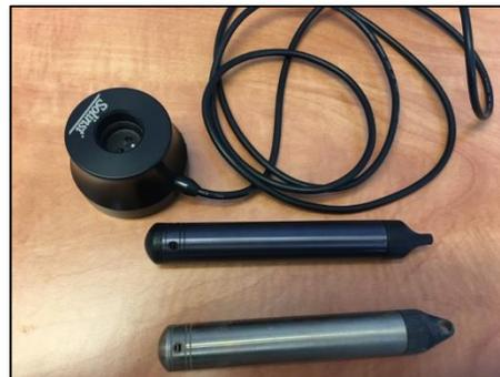
Figure 1. Pressure transducer dataloggers and optical reader.
