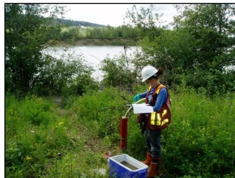
Figure 1. Well development using inertial lift for surge and over-pump method.
