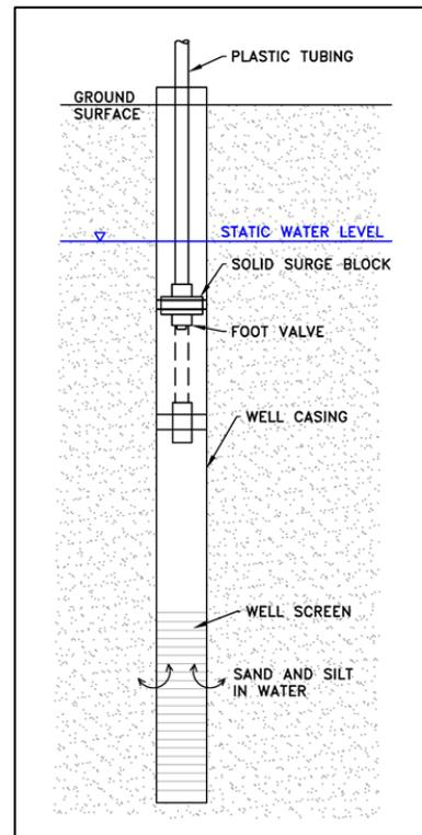
Figure 2. Schematic of inertial hand pump surging.
