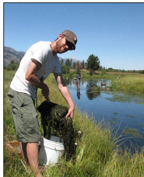
Figure 2. Aquatic plant sampling using rake toss from shore. Photos credit: Portland State University .
