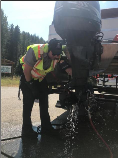
*Engine flush being performed by inspectors at the Yahk inspection station as part of the decontamination of a high risk pontoon boat.*
