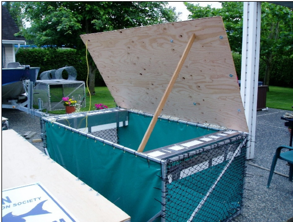
Photo 1. Sturgeon holding pens. Holding pen volume was 2718 L , and measured 2.43 m long, 1.22 m wide (front to back) and 0.91 m deep (top to bottom), or 8x4x3 feet.
