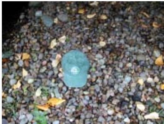
Figure 4c. Gravel material placed within the culvert.
