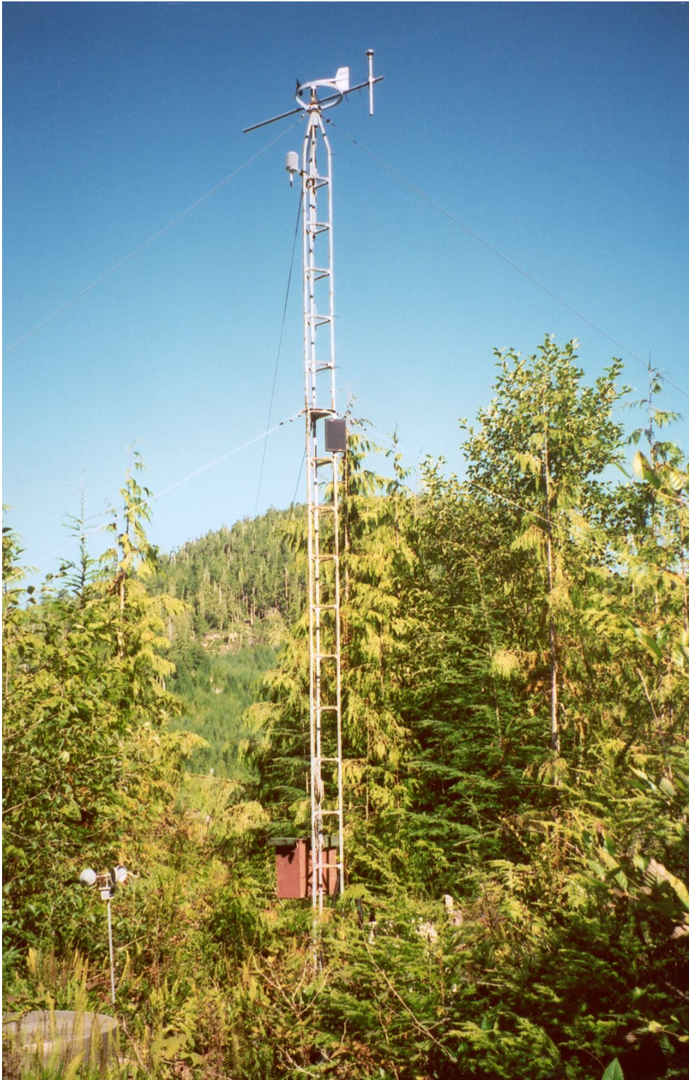
Climate stations located at several sites and elevations monitor variables such as air temperature, solar radiation, precipitation, relative humidity, wind speed, and wind direction. Shown is climate station A.
