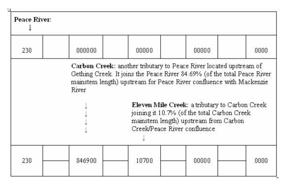
Figure 10 - Explanation of the Eleven Mile Creek Watershed Code, a Tributary to Carbon Creek in the Peace River Watershed
