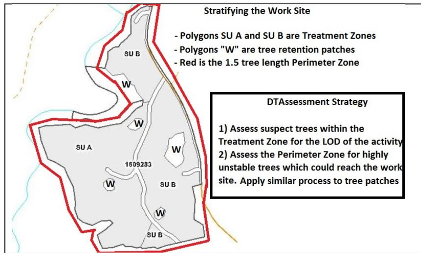
**Figure 1:** Example of stratifying a work site to define the scope of the DT assessment.
