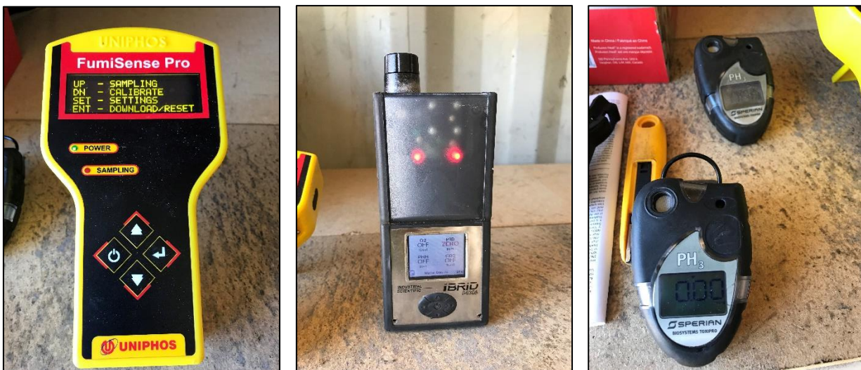
Figure 10. Example of gas detection and monitoring devices used in fumigations
