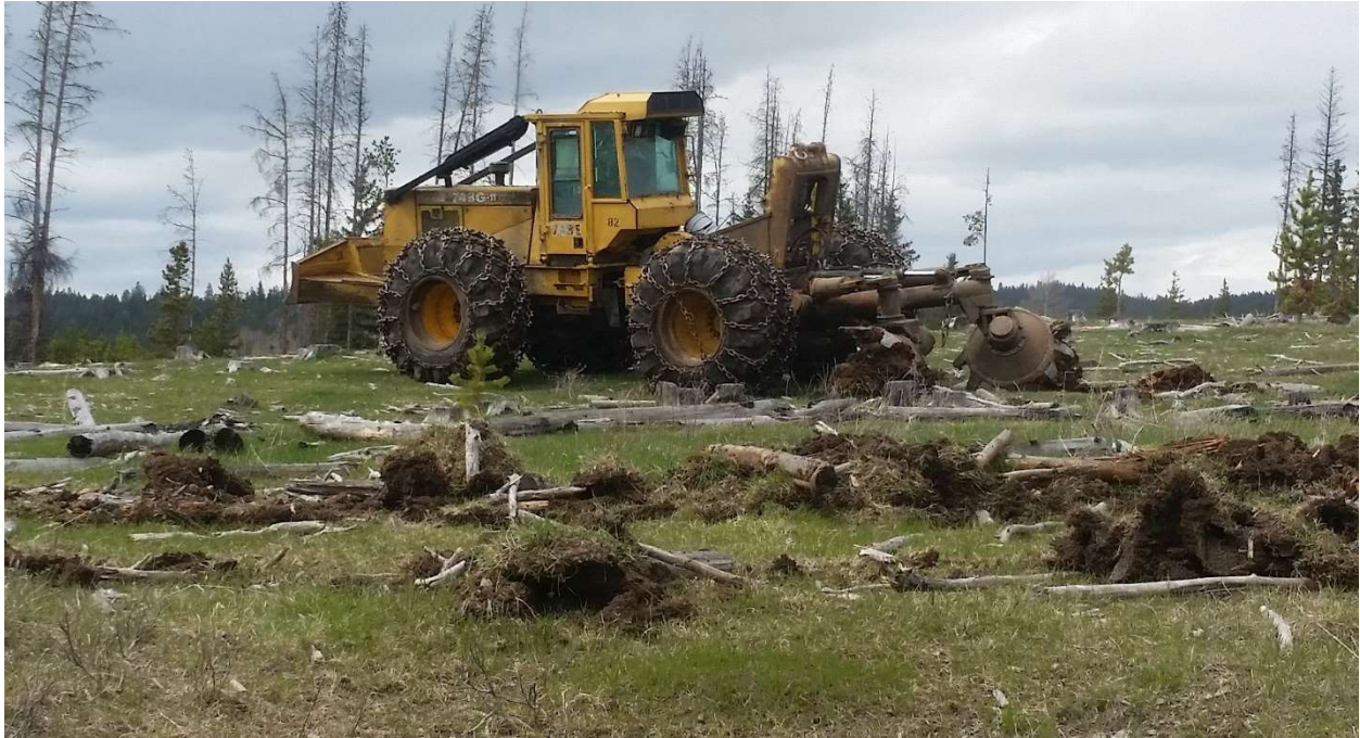
Photo 13. Example of poor disturbance on single pass disc trenching. Note the flat, compact soils which are very difficult to provide adequate disturbance. Photo provided by Clayton Franz
