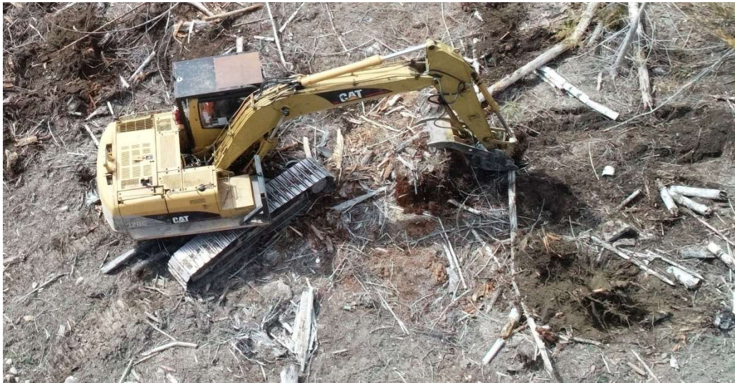
Photo 7. Excavator used for stumping and raised screefs. Photo provided by Jillian Schochter
