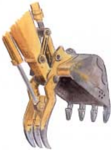
Standard bucket with extended teeth and live thumb
