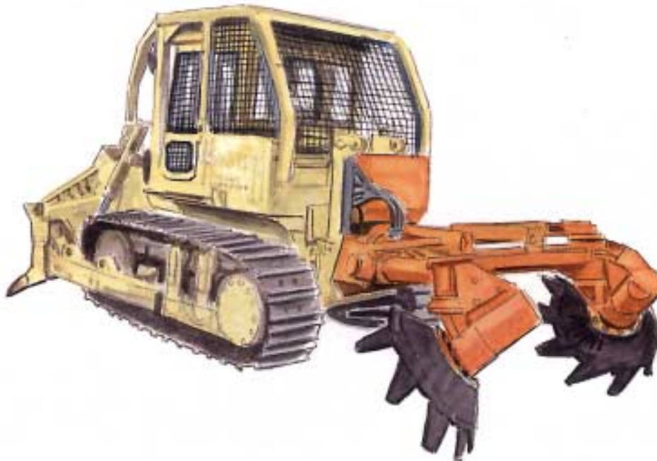
TTS powered-disc trencher mounted on a crawler
