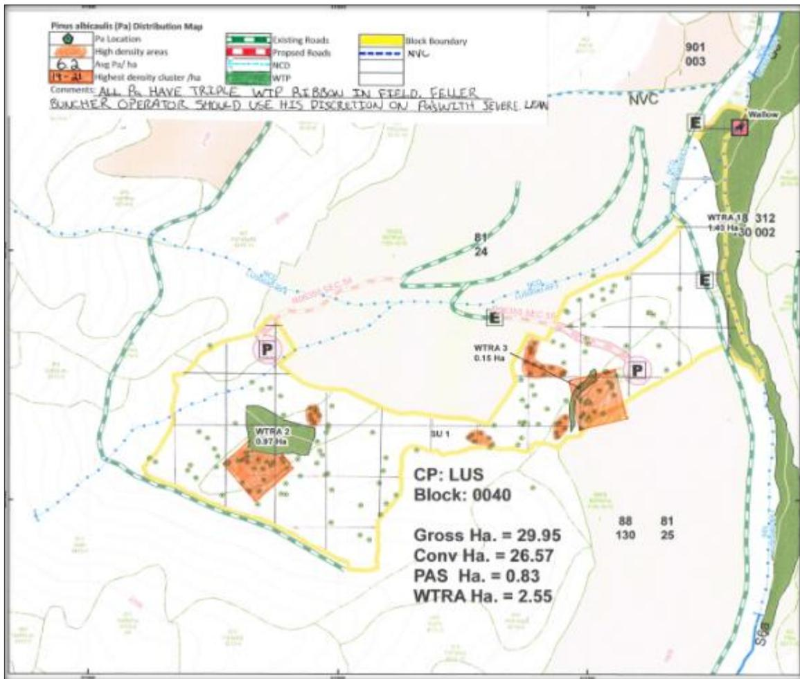
Figure 24. Map showing whitebark mapped during cutblock layout. Green areas are no-harvest reserves; orange blocks are high density whitebark pine; note tree marking and machinery operator notes. Layout map courtesy of Canfor (2016).
