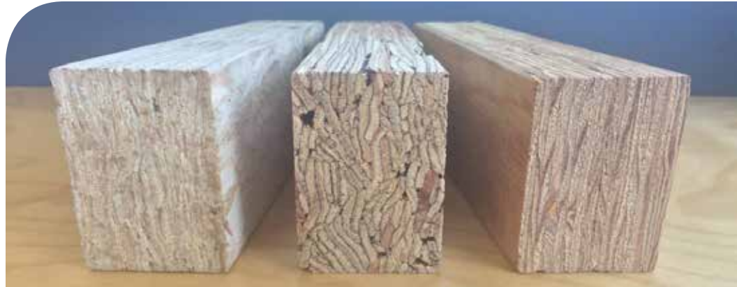
Structural composite lumber products. From left-to-right: laminated strand lumber (LSL), parallel strand lumber (PSL), and laminated veneer lumber (LVL) (Image courtesy of Tom Joyce).
