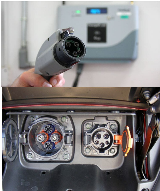
Top Left: Level 1 Charger (J-1772 plug). Top Middle: Level 2 Charger (J-1772 plug). Top Right: Level 3 DC Fast Charger (CHAdeMO plug). Bottom Left: Shows a vehicle charge port with CHAdeMO port on the left and J-1772 port on the right. Note that Tesla uses completely different plugs, not pictured here, which can use adapters to work with these standard adapters.
