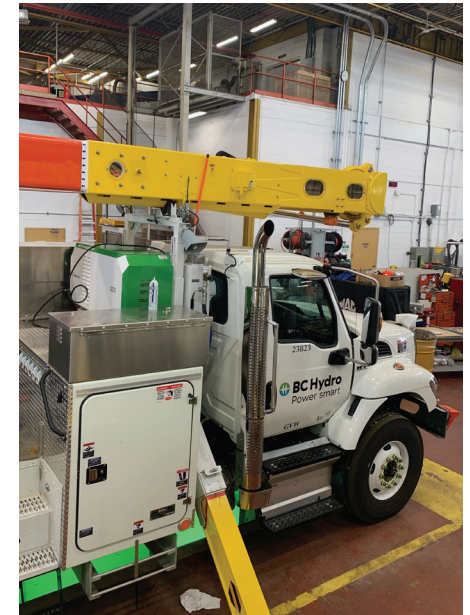
Electric power takeoff (ePTO) system that powers the boom and auxiliary functions on bucket trucks
