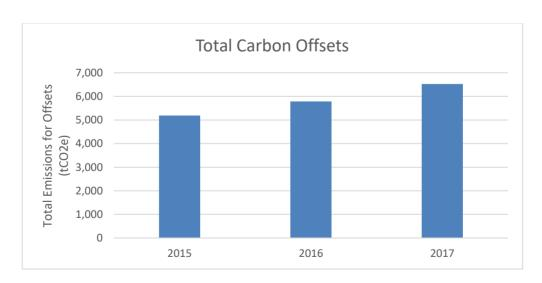
The 2017 carbon emissions were higher than 2016 due to colder weather experienced. There was a 20% increase in the number of heating degree days in 2017 than in 2016. This caused an increase of natural gas consumption which is responsible for most of the increase.
