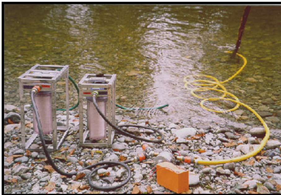
Figure 1. Configuration of apparatus for splitting G/C samples.
