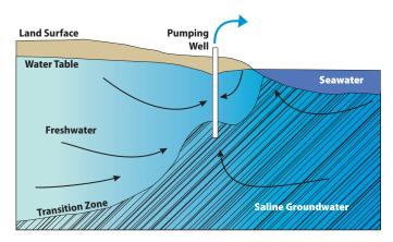
**Figure 2:** Pumping or other disturbances (e.g. sea level rise, reduced recharge) can lead to upconing or inland movement of the freshwater-saltwater interface. If a single well is overpumped or multiple wells are pumping, a large area of the aquifer may be impacted by salinity.
