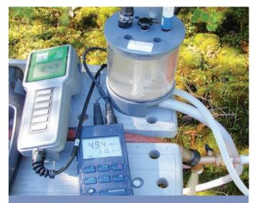
A hand-held meter used to measure specific conductivity (shown above).
