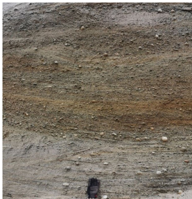
Figure 2: Photo of glaciofluvial sand and gravel comprising AQ751 exposed in an excavation in a gravel pit off Heriot Bay Road.
