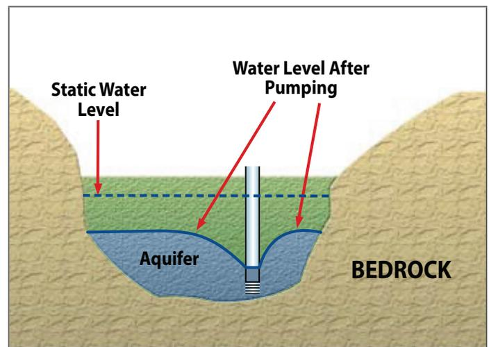
**FIGURE 8** *Drawdown behaviour in small unconsolidated unconfined aquifer bounded by bedrock.*
