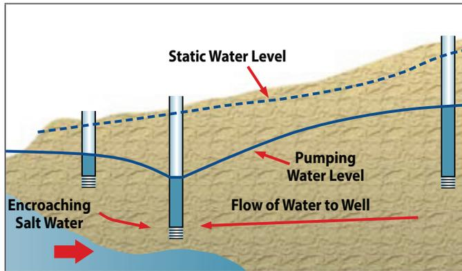
**FIGURE 9** Pumping test of a well adjacent to the ocean.
