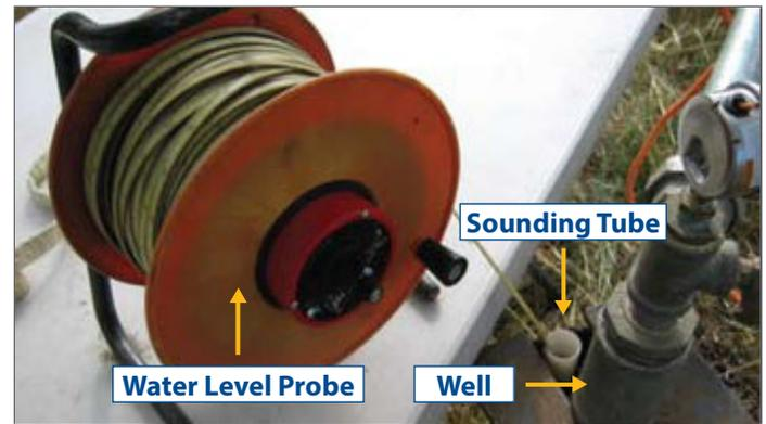
**FIGURE 5** Water level measurement using water level probe and sounding tube.
