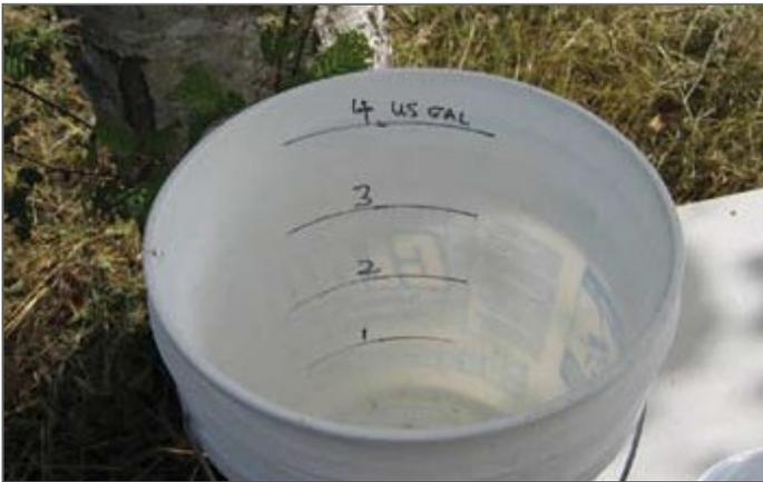
**FIGURE 4** A five gallon bucket and a stop watch can be used to estimate low pumping rates.
