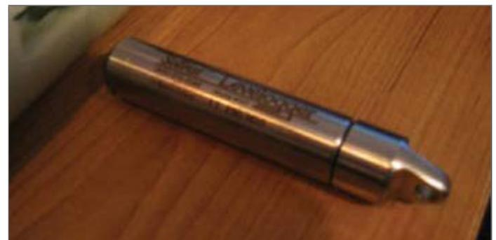
**FIGURE 6** A pressure transducer can be used for automatic measurement and recording of water level and temperature, specific conductance or other parameters during the pumping test.
