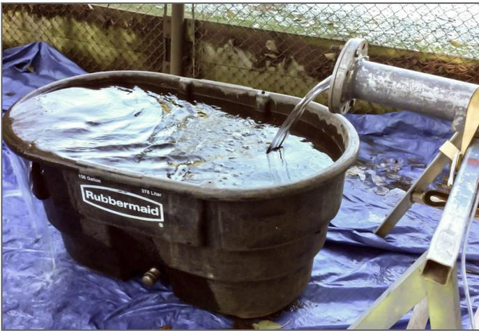
**FIGURE 7** *Water discharge during a pumping test*
