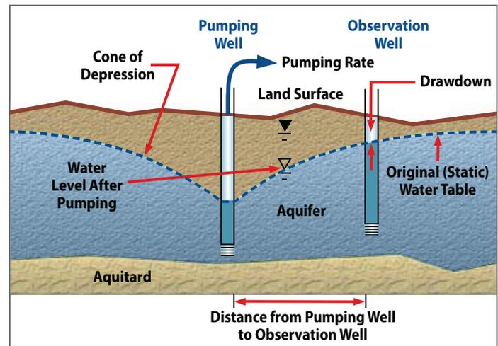
**FIGURE 1** This figure shows the impact of a pumping well on the water table and a neighbouring well (observation well) in an unconfined aquifer. As the water is pumped from the well, the original or static water level lowers, i.e., drawdown occurs in the well. A cone of depression is formed in the aquifer around the pumping well as the water level declines due to pumping. Note that drawdown in the observation well is much less than in the pumping well.
