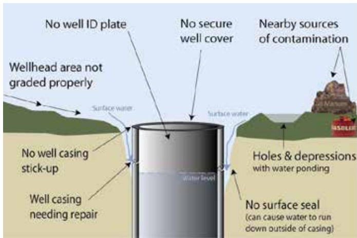
FIGURE 7 Common dug well issues
