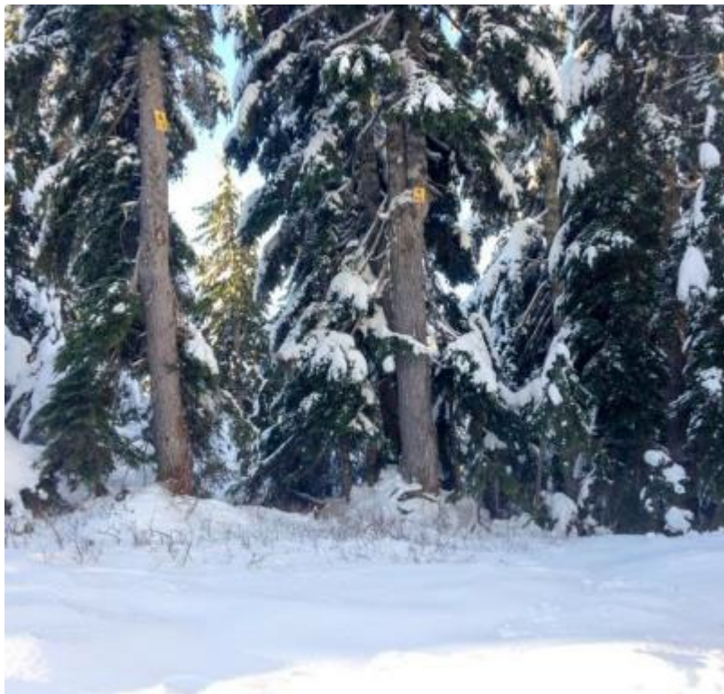
Figure 8: Sampling station with 2 reference plates - installed above the maximum snowpack - from which the sampling location can be triangulated.
