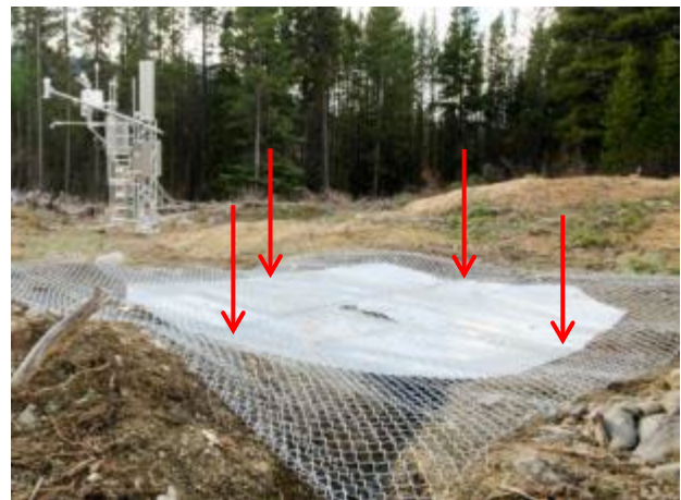
Figure 27: 4-point verification at a snow pillow
