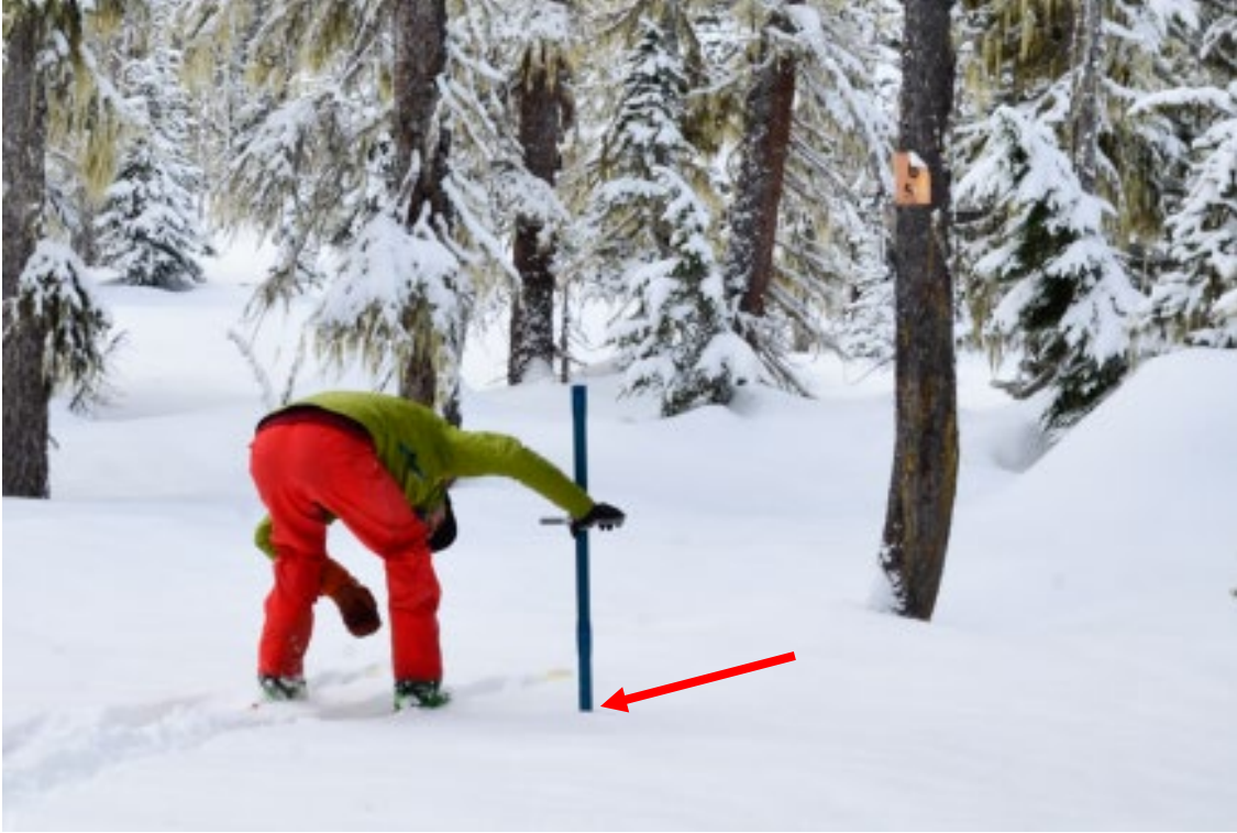
Figure 17: Reading the depth of snow with dirt plug.
