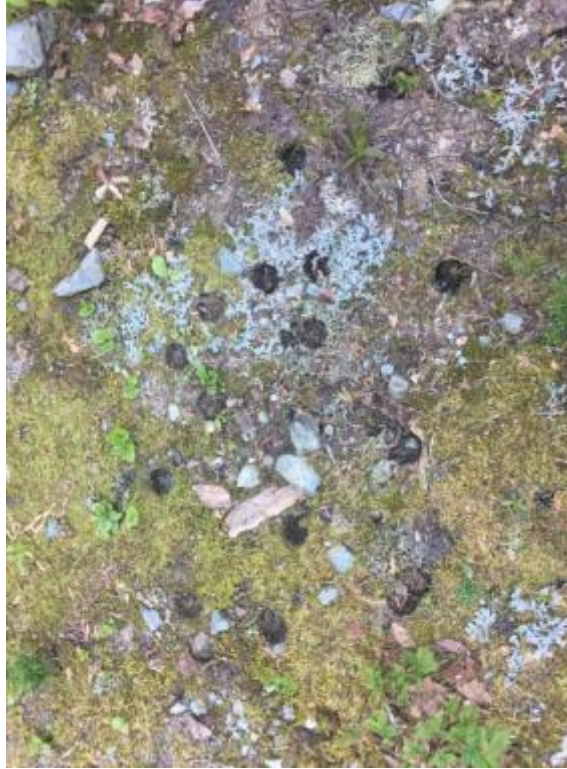
Figure 9: Core cutter marks and evidence of sampling within a 1.5 m radius.
