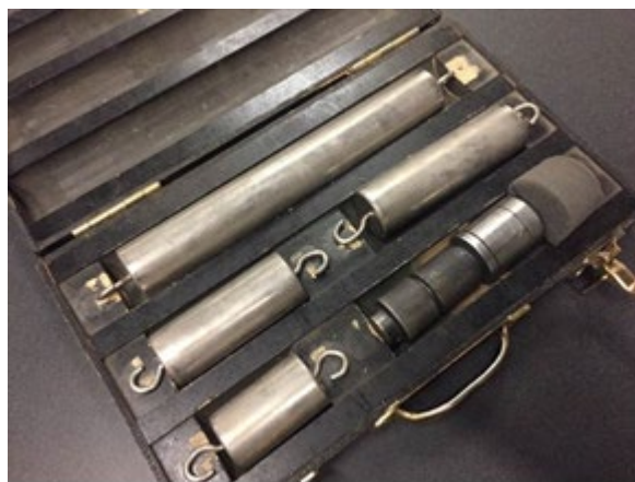
Figure 4: Scale calibration weights
