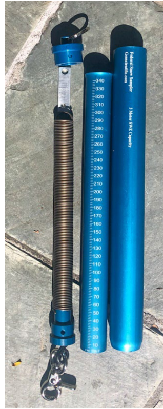
Figure 2: Inner workings of a scale
