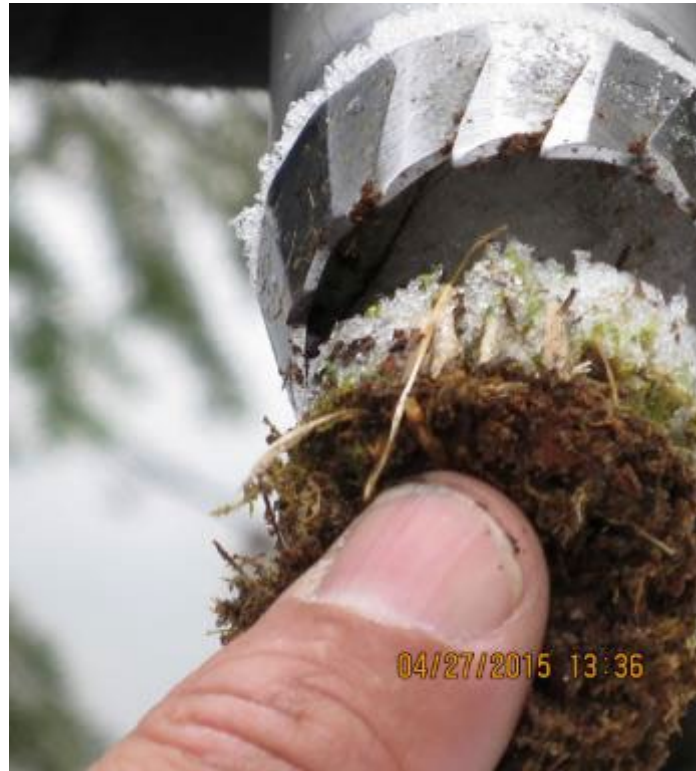
Figure 21: Removal of the dirt plug.
