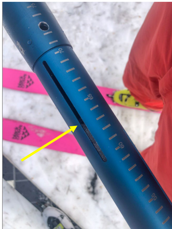
Figure 17: Reading the depth of snow with dirt plug.
