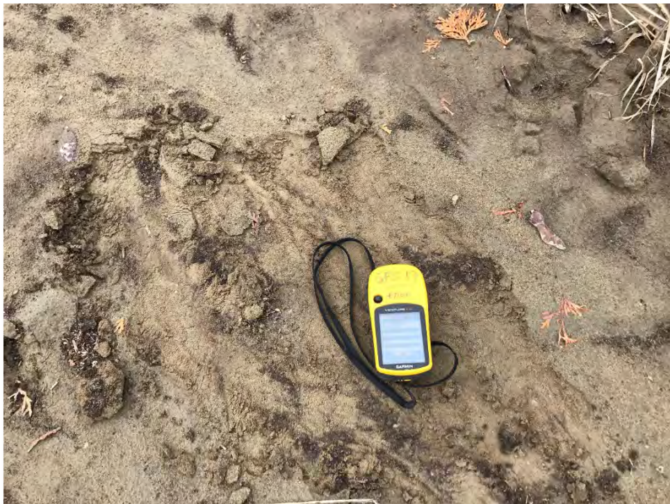
Photograph 4: P-SS22-02: SAND, fine grained, trace silt, brown, loose, trace rootlets, damp.
