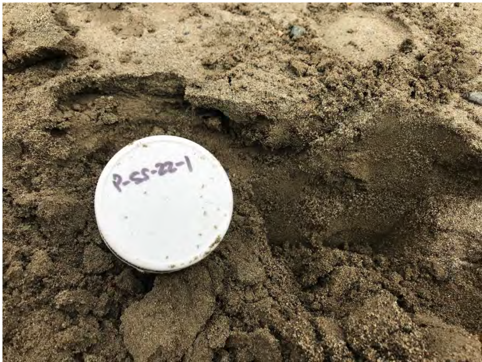
Photograph 2: P-SS22-01: SAND, fine-medium grained, trace silt, brown, loose, trace rootlets, damp.
