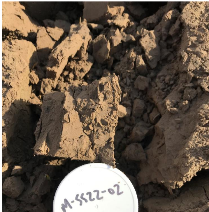
Photograph 2: M-SS22-02: SILT, some clay, some fine grained sand, brown, trace organics, moist.
