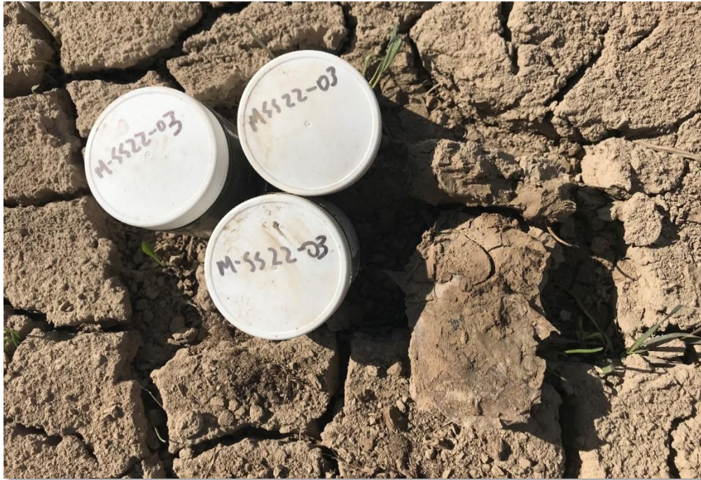
Photograph 5: M-SS22-03: SILT, some clay, some fine grained sand, brown, trace organics, moist.
