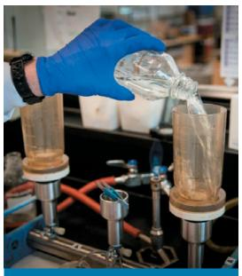
Rinsing the filter housing for membrane filtration. Photo credit: BC Centre for Disease Control - Public Health Laboratory.
