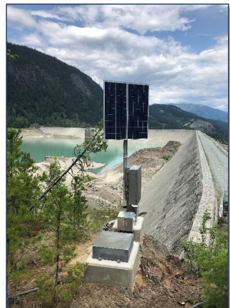
Photo 2: Solar-powered, seismic monitoring station, using a nanometrics broadband monitoring station, for hard rock
