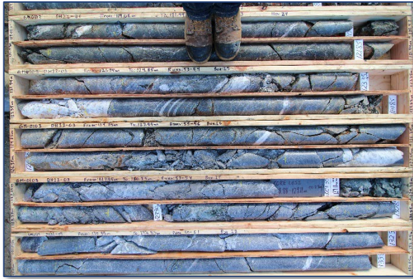
Photo 4: Drill core samples from a dam foundation.
