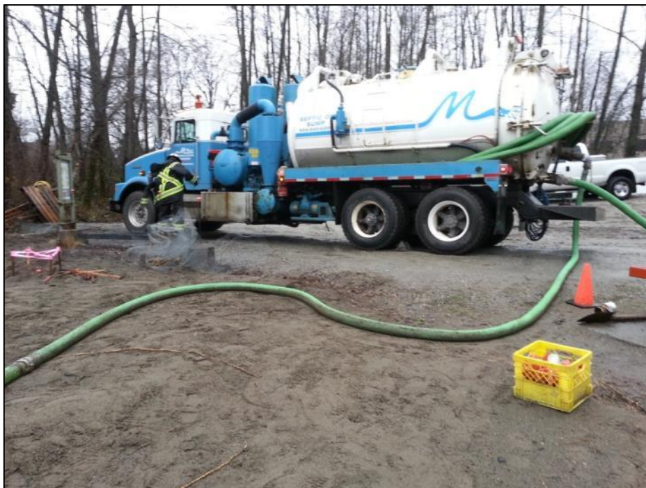
Photograph 18: Vacuum truck used in the recovery of coal
