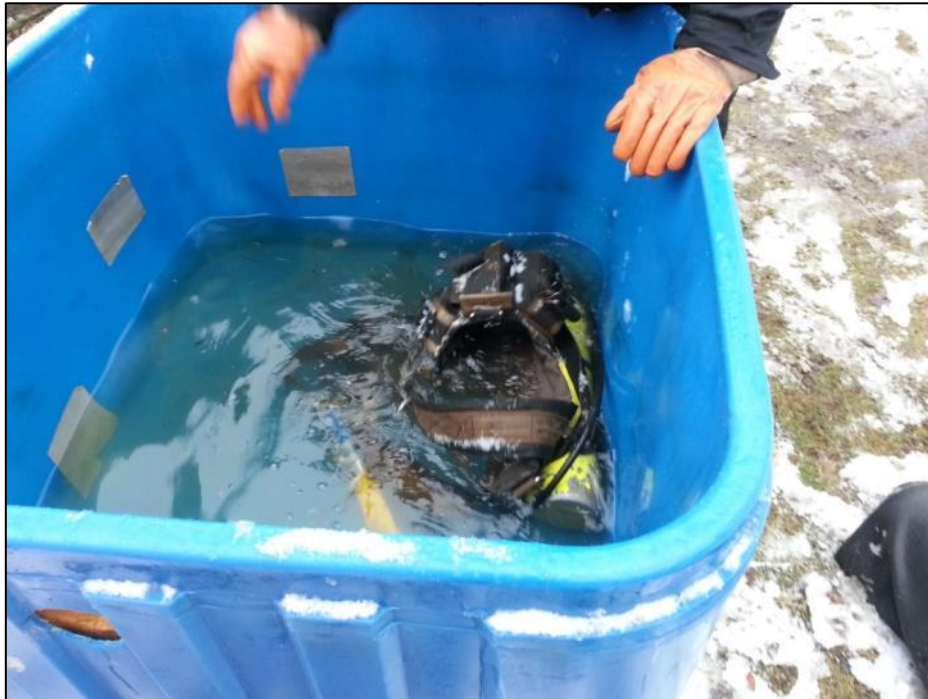
Photograph 13: All equipment (including diver gear shown here) was scrubbed and disinfected with bleach prior to use in the recovery area
