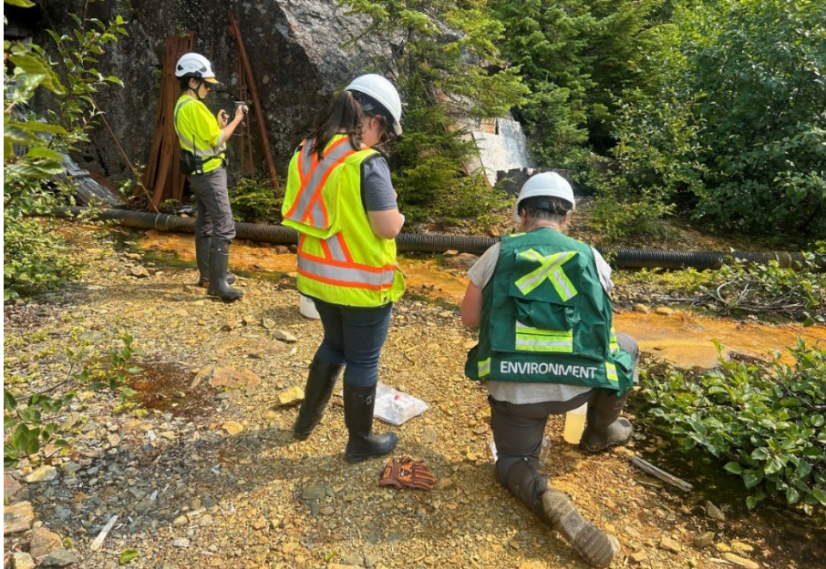
Figure7: Discharge sampling being conducted at the 5400 portal.
