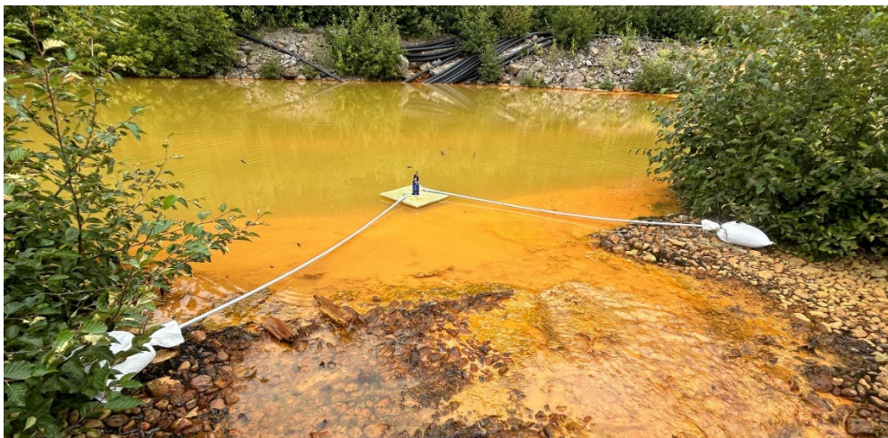
Figure 8: A sonde installed at a collecting pond for continuous water discharge quality monitoring.
