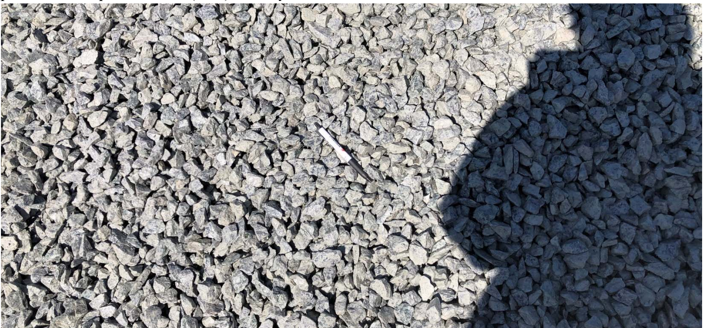
Picture # 2: Close up photo of the proposed clear crush drainage gravel. Pen for scale.
