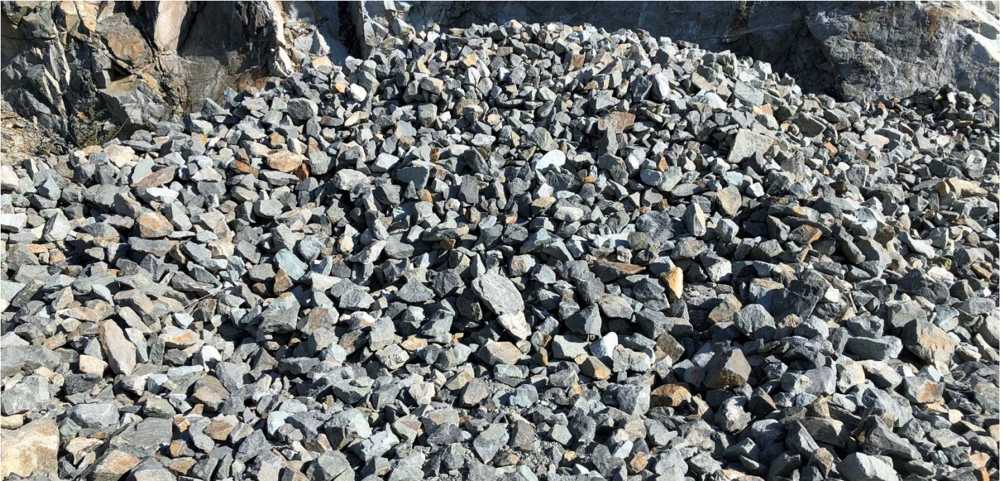
Picture #5: SHA inspected the stockpile of blast rock. SHA inspection confirmed that the material appears suitable for proposed use of backfill in the soak away trench.
