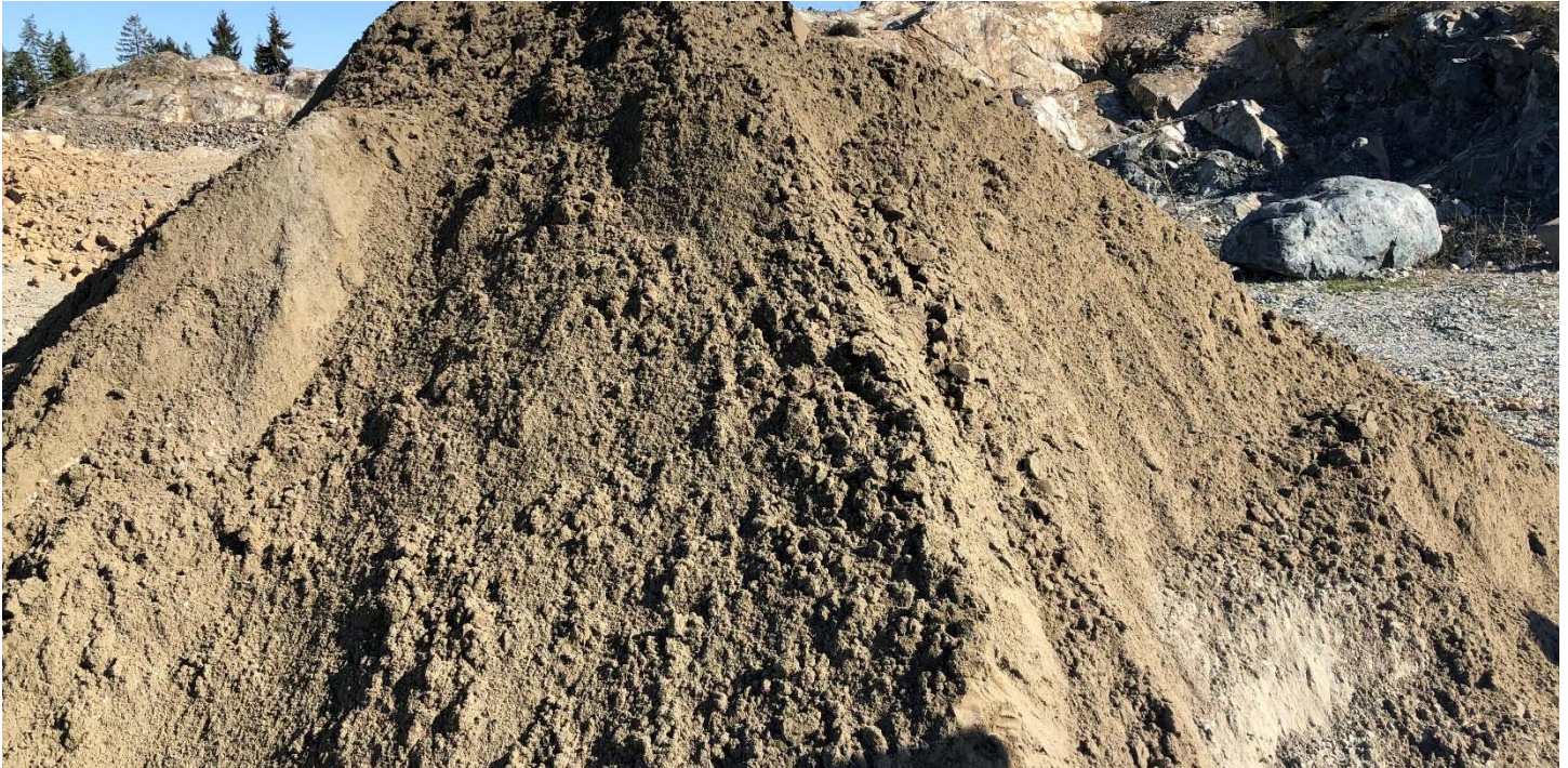
Picture # 3: SHA visually inspected the stockpile of proposed sand. SHA inspection confirmed that the material is a fine sand that appears suitable for proposed use as the 50mm thick sand layer above the PEA geomembrane.
