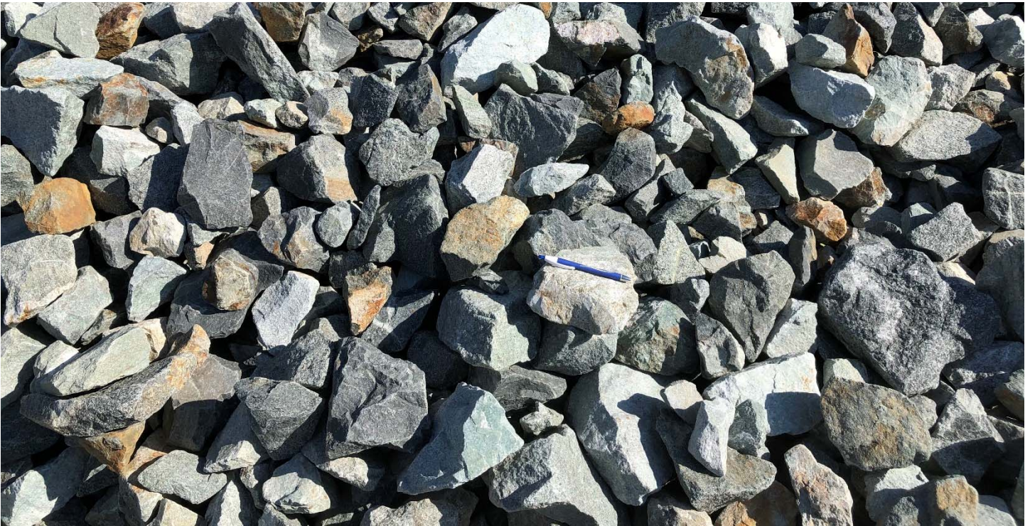
Picture #6: Close up of blast rock stockpile. Pen for scale.
