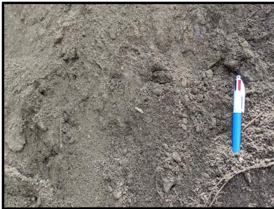
Picture # 2: View of soils from 2251 Bear Mountain Parkway. Generally sandy with some gravel and larger angular cobbles.
