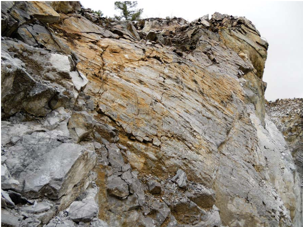
Photo 2: Entrained fragments and gouges along a fracture face in the Butler Quarry
