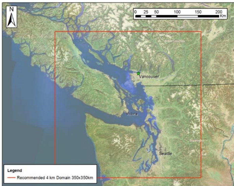
Figure 2-1. Example photochemical modelling domain (red box) centered over the LFV covering a 350 km square area with 88x88 grid cells at 4 km grid resolution.
