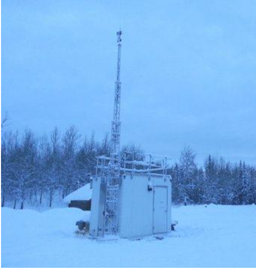
Figure 2 An air quality monitoring trailer at Doig River, north of Fort St. John, one of three portable monitoring trailers operated as part of in the Northeast BC Air Quality Monitoring project from 2013 through 2017 .
