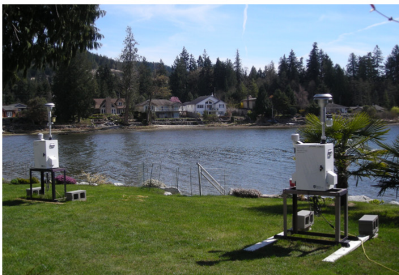
Figure 2. PM monitors in Sechelt. (a) Trail Bay Mall (TBM) monitoring site with dichot instrument, facing east; and (b) East Porpoise Bay (EPB) monitoring site with two Partisols, facing south.
