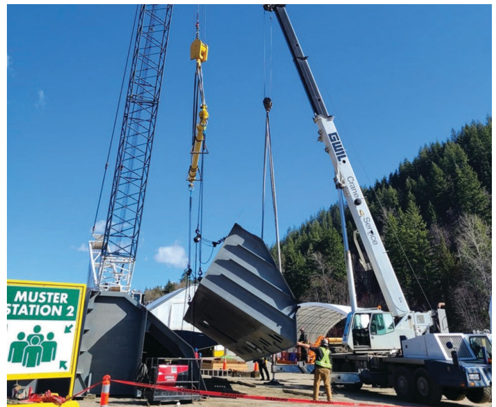
The crane in action—lifting a hull block from the assembly site to the drydock.
