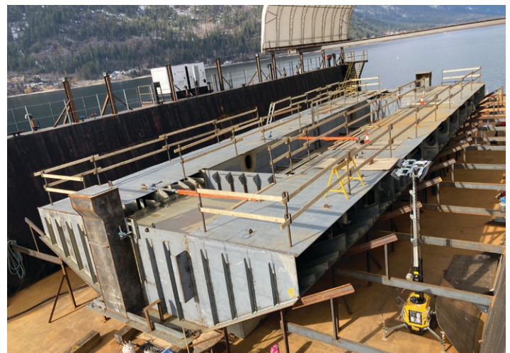
A view of the partially assembled hull in the drydock on the lakeshore.
