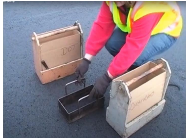
C2 - Placing sampling template at selected location on newly placed asphalt mat.
