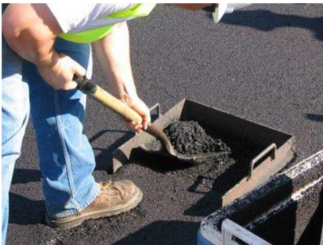
C7 - For bigger sampling template shovel can be used.
