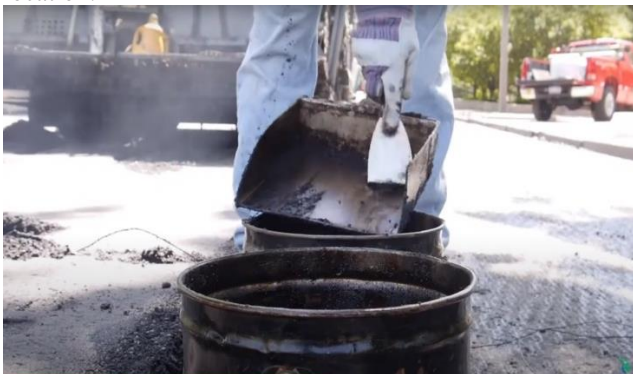
A3: Scraping off leftover asphalt mix/fines from the shovel into sample container.
