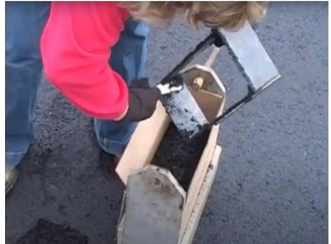
C6 - Scraping off leftover asphalt mix/fines from the template into sample container.
