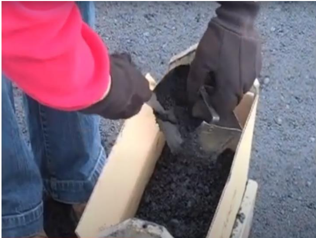
C5 - Scraping off leftover asphalt mix/fines from the scoop into sample container.
