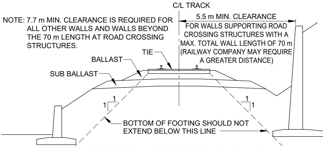
NOTE: 7.7 m MIN. CLEARANCE IS REQUIRED FOR ALL OTHER WALLS AND WALLS BEYOND THE 70 m LENGTH AT ROAD CROSSING STRUCTURES.
