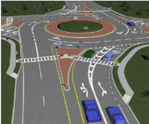
Figure 740.E Example of Entry Lanes to Accommodate Truck Over Tracking (from New York DoT)
