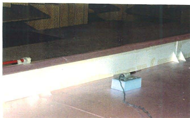
Figure 4.2; Scale Model Test Setup for 4 m Wall (3 m above Pavement).
