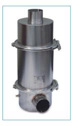
Diesel oxidation catalysts can reduce emissions of diesel particulate matter (PM) by 20 percent, hydrocarbons by 50 percent and carbon monoxide (CO) by approximately 40 percent, based on regular diesel fuel. They can be installed on off-road equipment and on diesel equipment that must operate within enclosed spaces (e.g. mines, buildings). A DOC can operate on virtually any engine on any duty cycle, and, as a passive device, is typically maintenance free.
