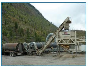
Typical portable asphalt plant
