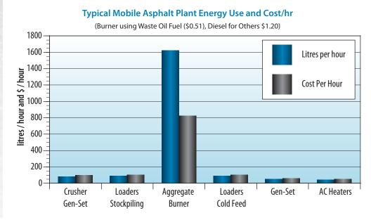
A typical portable asphalt plant uses waste oil for the dryer burner, off-road diesel for the loaders, gen-sets and AC heaters and on-road diesel for the haul trucks. The aggregate burner is by far the largest energy consumer and, hence, the largest source of GHG emissions (see figure on previous page).
