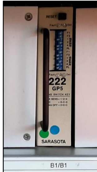
Figure 20. Typical Pre-emption Card Label
