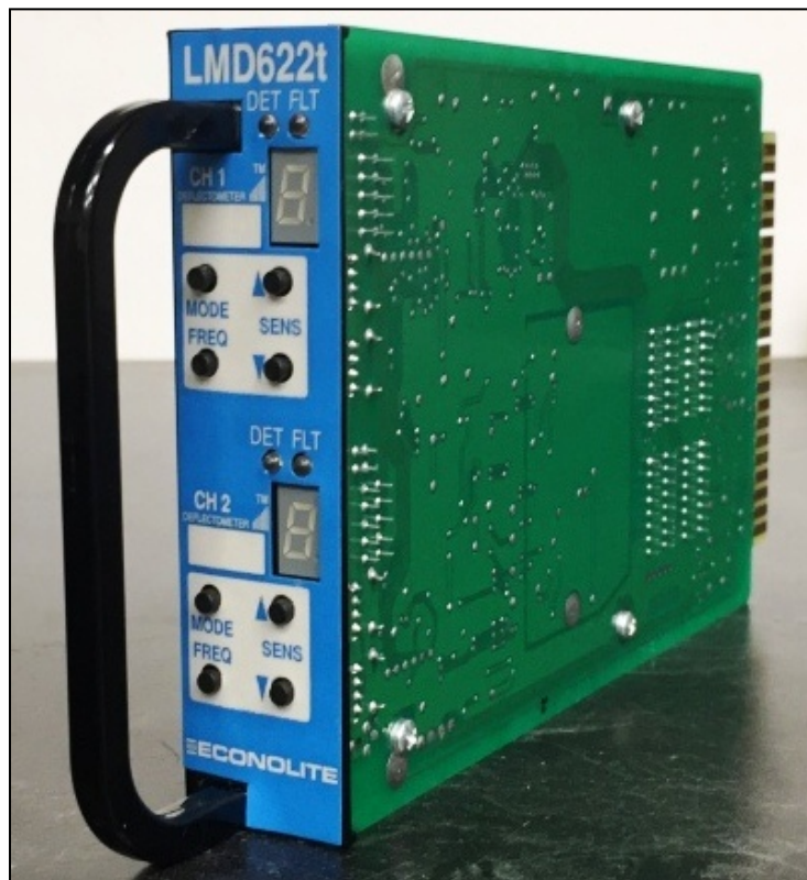
Figure 31. Typical Ministry Loop Detector
