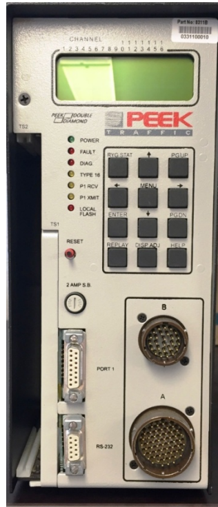
Figure 28. The Peek Traffic Double Diamond Malfunction Management Unit
