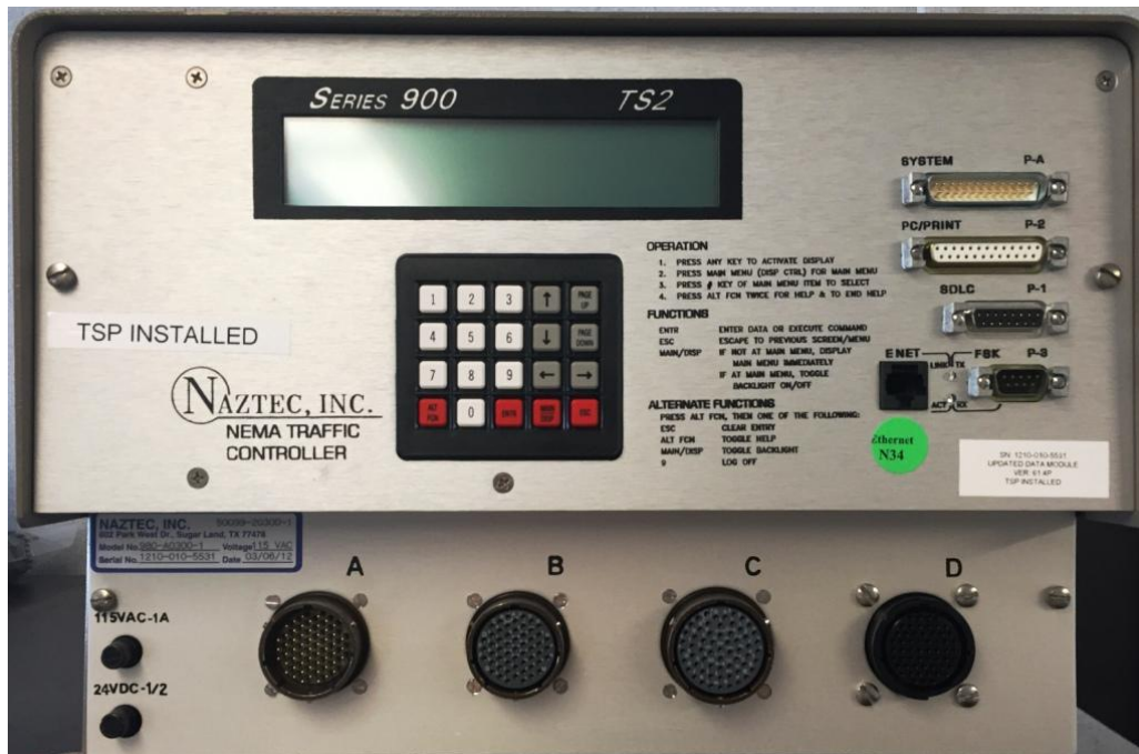
Figure 24. The Trafficware/Naztec 980 Type 2 Controller Unit
