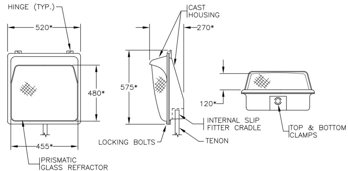
250W M.V. TYPE B SIGN LUMINAIRE (REFRACTOR STYLE)
